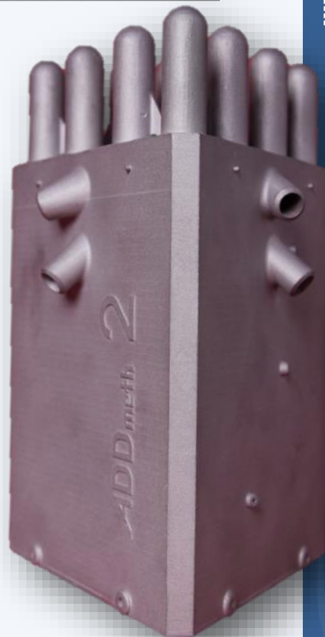
metal printed 20 kW up-scale ADDmeth2 ready for test rig integration
