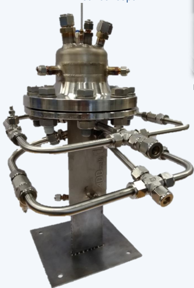
ADDmeth1 with fittings and piping for reactants, product gas, cooling and instrumentation
